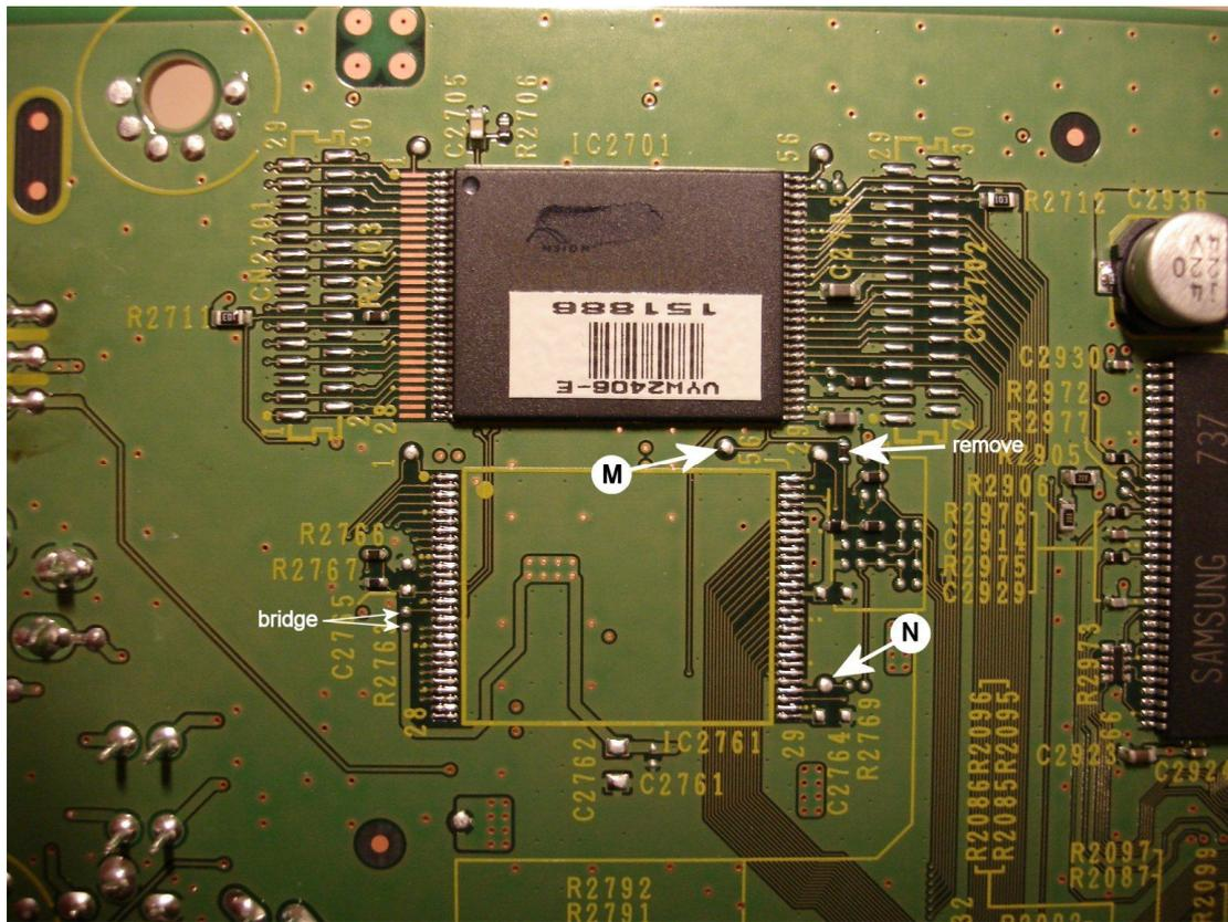
Install the supplied Flash chip at the empty spot on the board (IC2761).
