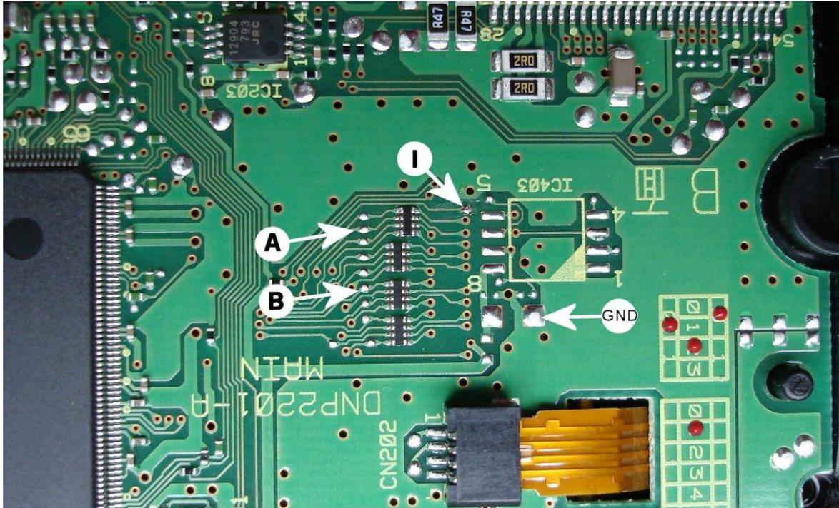
Solder wires from point A, B, I and GND to the corresponding points on the Logic board.
