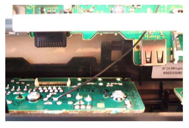
When re-fitting the front panel check that all 7 plastic clips are fully in place, otherwise the electrical connectors may not contact correctly.
