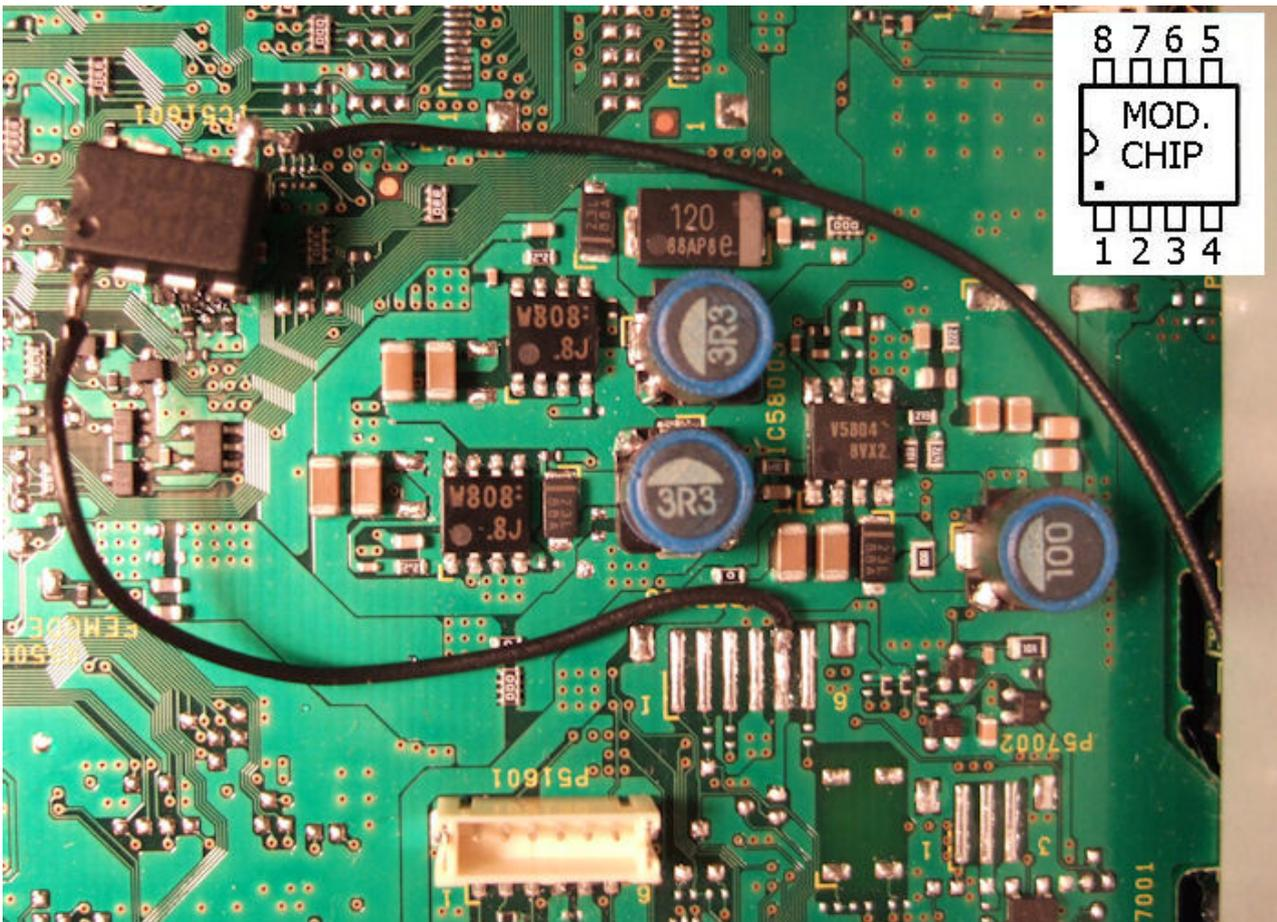
If you're not confident with the "piggy-back" fitting method just use wires to connect all 6 pins of the mod. chip.
