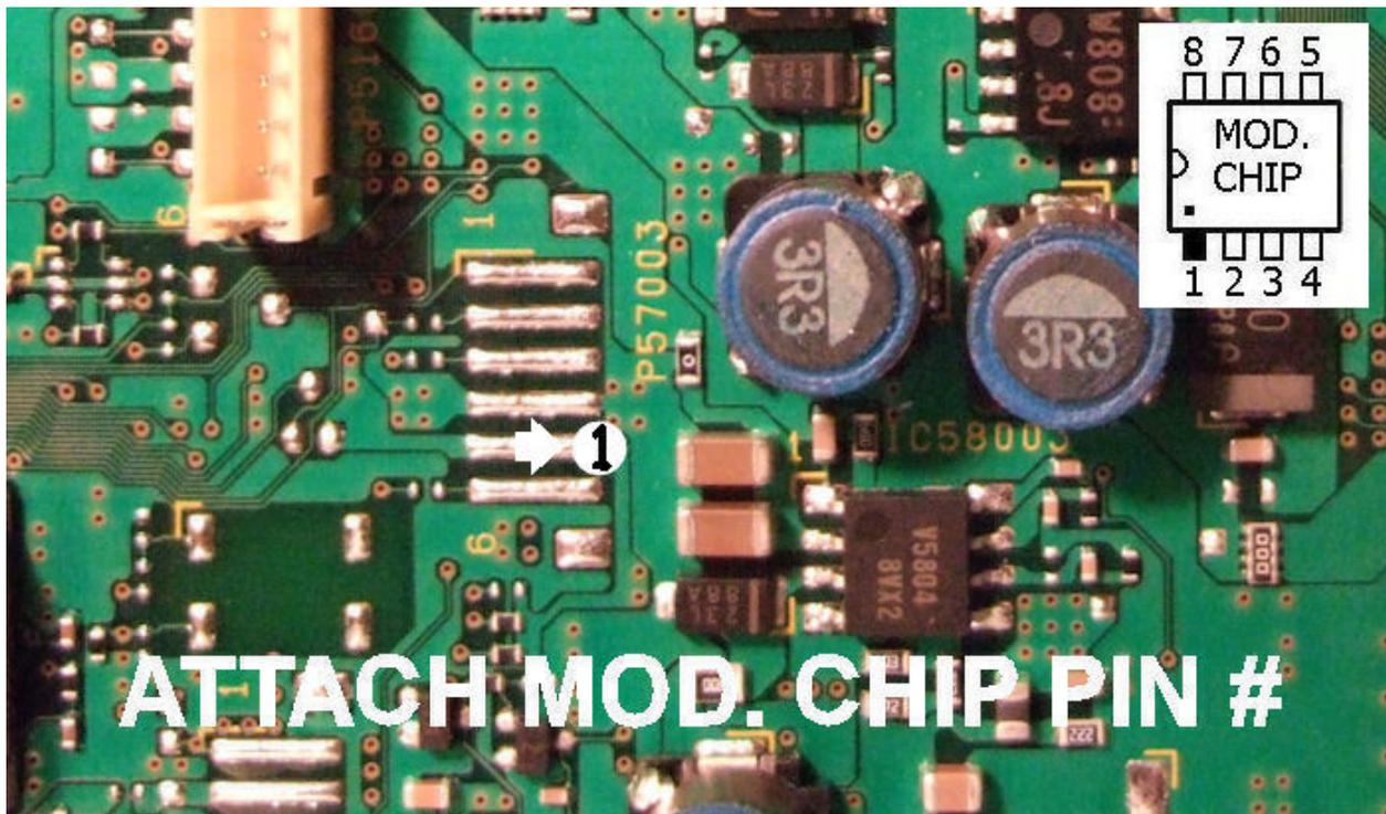
Mod. chip pins #2, #3, #4 and #8 should be connected to the small 8 pin chip as shown.
