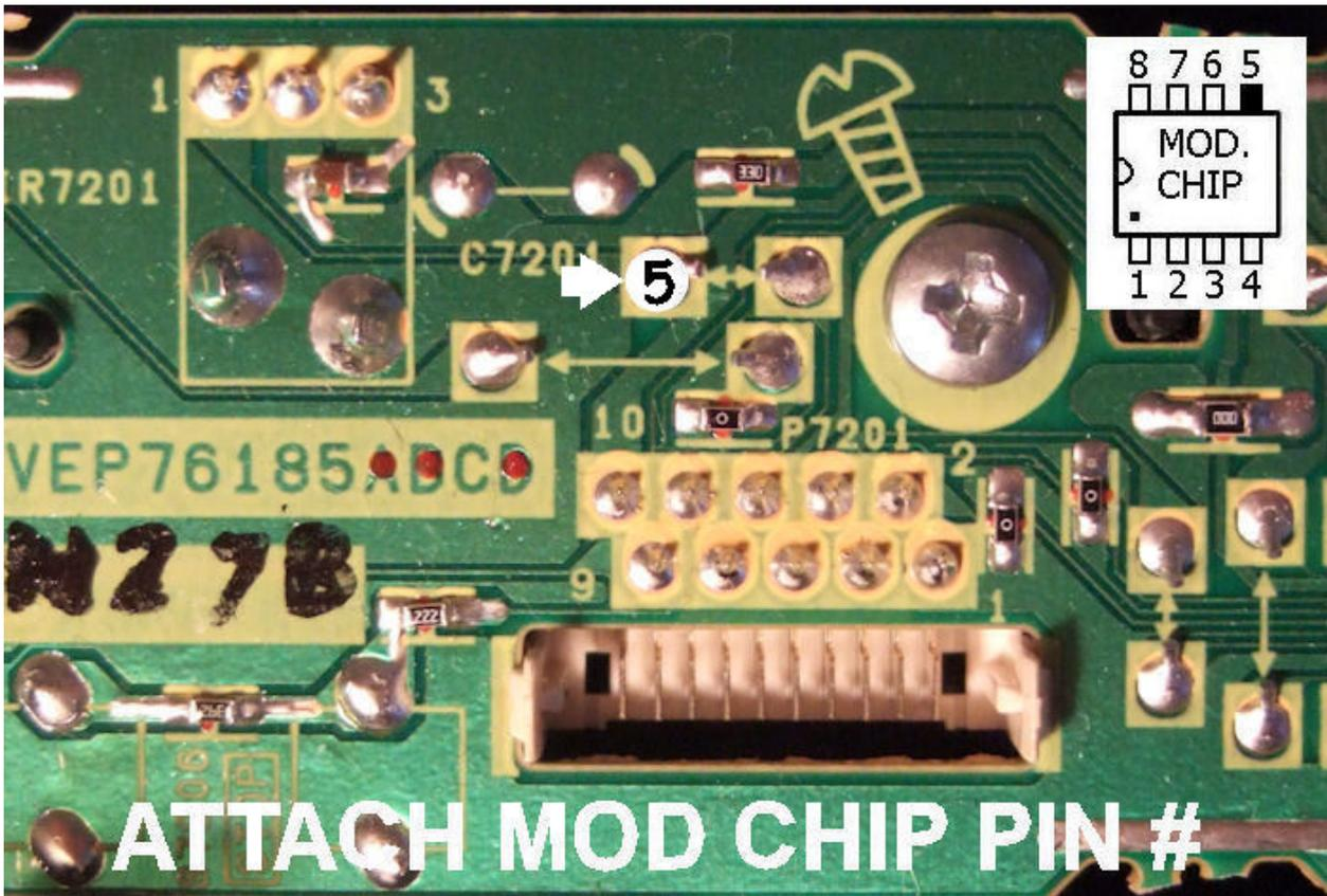
Bring the wire for mod. chip pin #5 in under the metal plate at the front of the player, ensuring that it doesn't block the connector shown at the left side.
