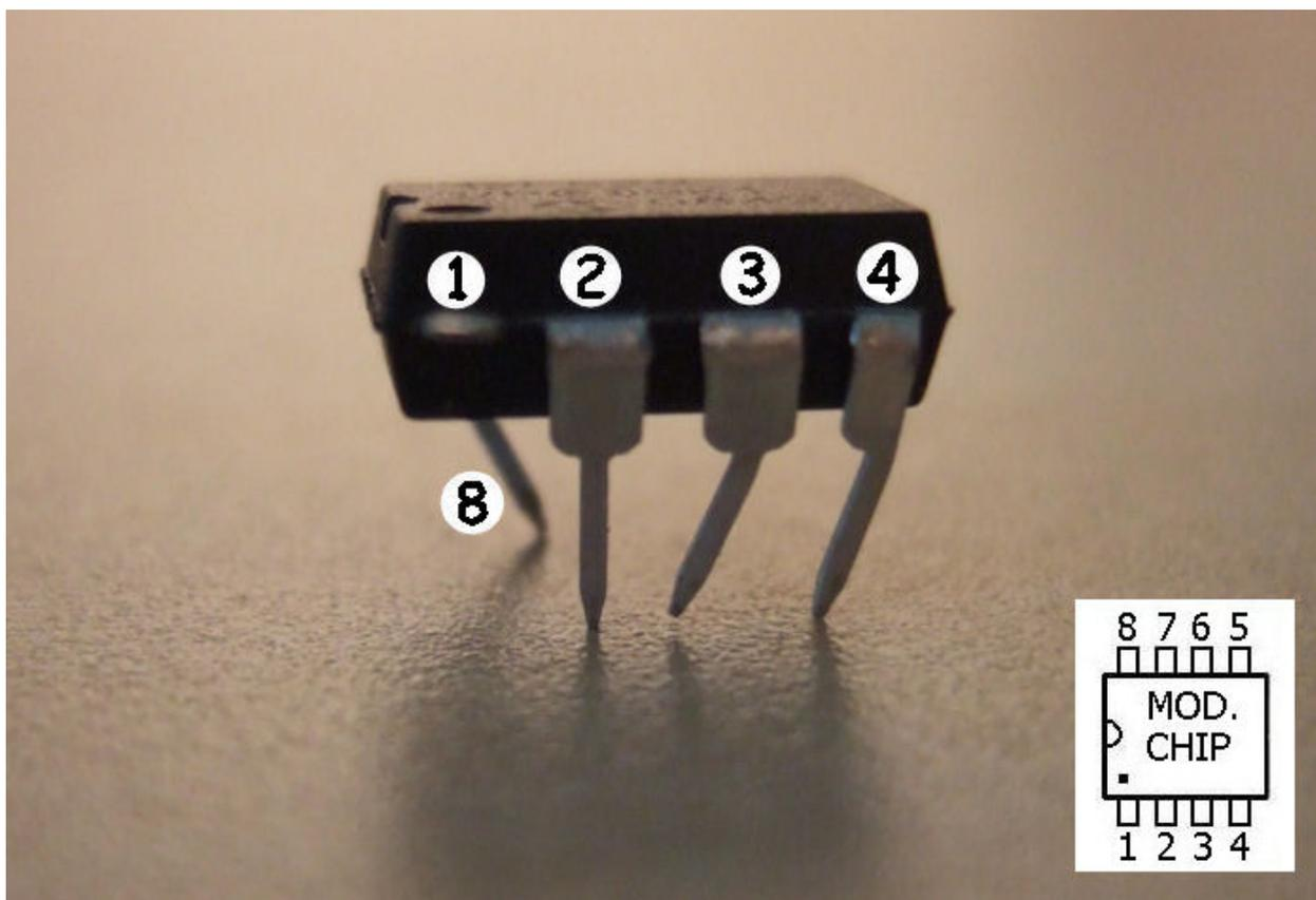
Bend the pins into position and then hold it against the chip on the board to make sure they are lined up correctly. Once all the pins are lined up solder pin #8 first, then you can carefully position the mod. chip by rotating it slightly and solder pins #2, #3 and #4.
