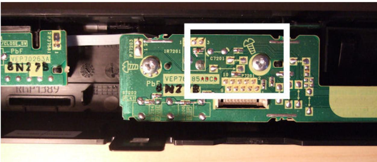
Connect pin #5 to the point on the front panel PCB shown below.
