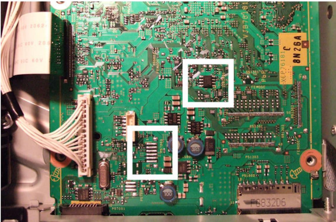
6 pins on the mod. chip are used in total, #1, #2, #3, #4 and #8 connect to the main board and #5 to the rear of the front panel.
